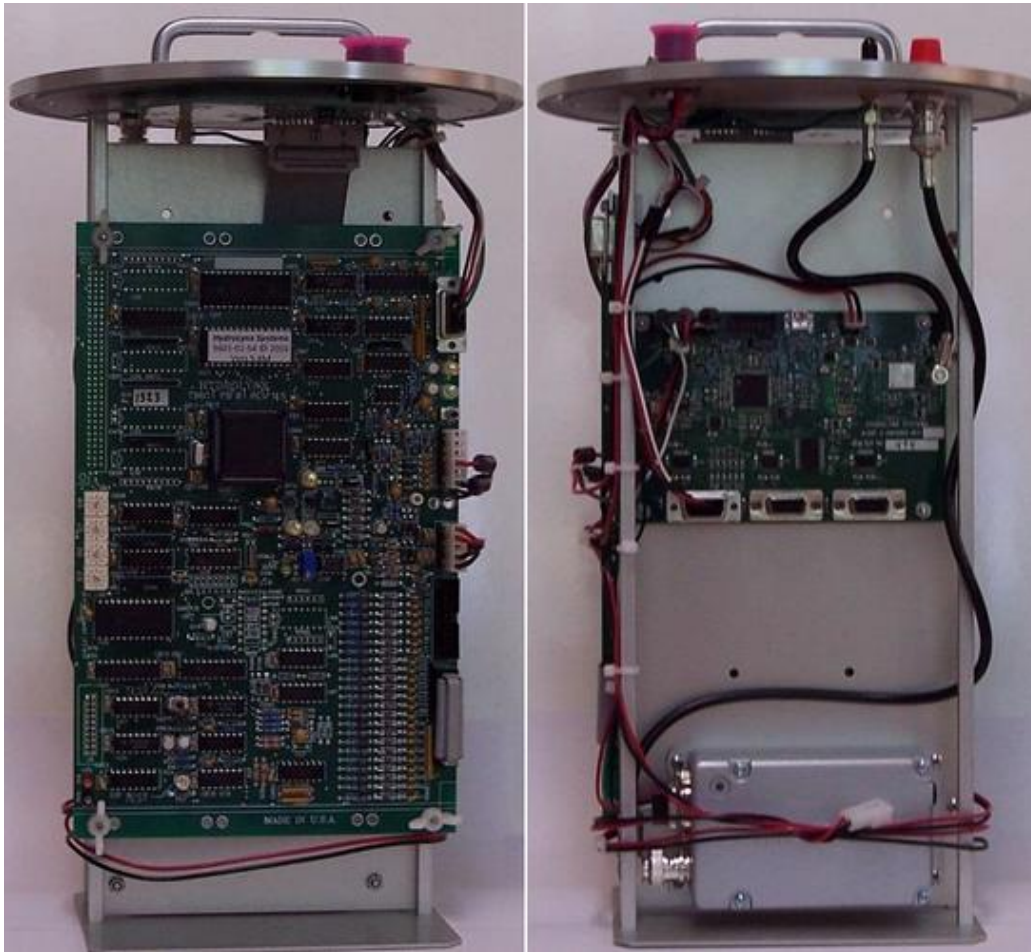
Model 5096/A2 — original 5096 PCB (left) and ALERT2 upgraded unit with encoder installed (right)
